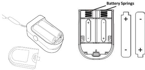
Figure 3 Batteries installation
