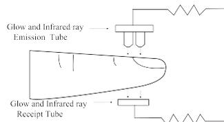
Figure 1 Operating principle
